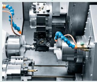
Superimposed cycle is simultaneous machining through overlapping control between L-spindle and R-spindle.
