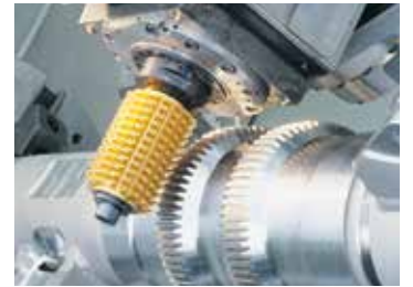
Hobbing of gear teeth (Flanx-Hob)
