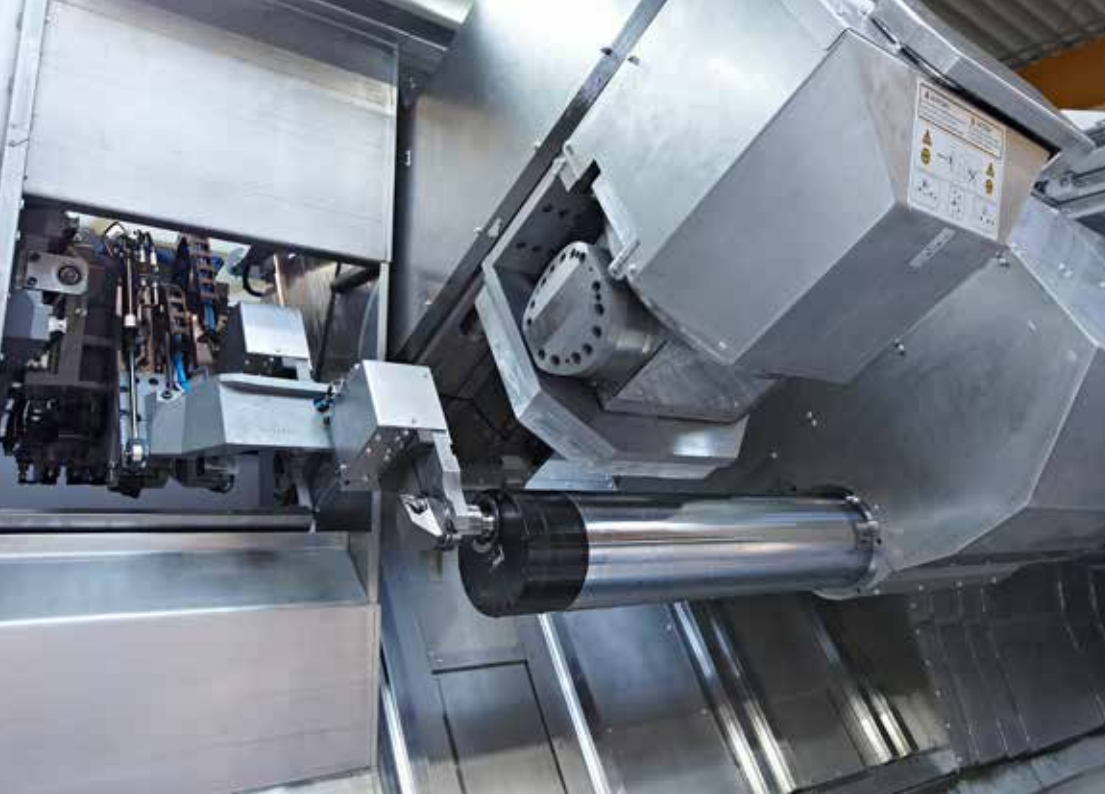
Tool change on boring bar
