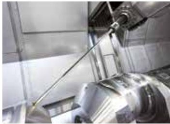
➤ Deep hole drilling
