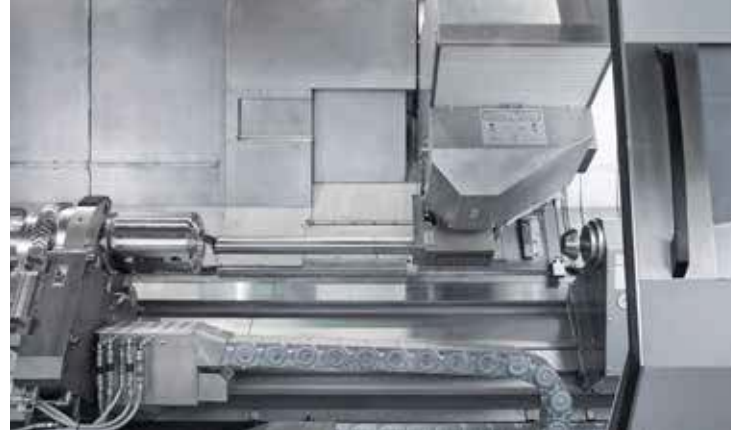
Internal machining with damped boring bar
