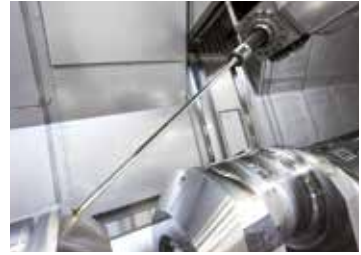
Deep hole drilling
