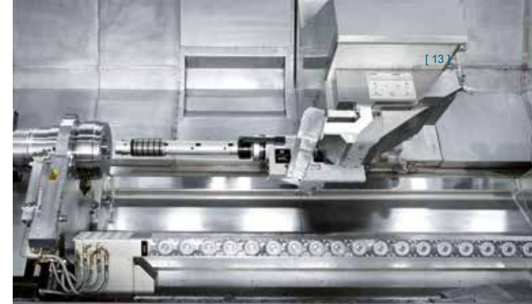
CNC special contour boring bar (radial feed out using the U-axis)
