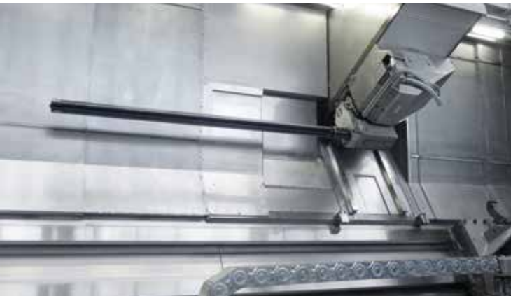
Deep hole drilling with automatic coolant docking
