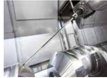
Deep hole drilling
