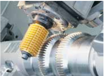
Hobbing of gear teeth (Flanx-Hob)
