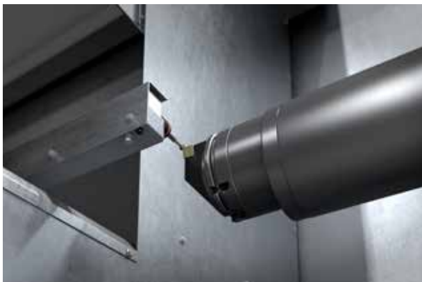
Tool control in the working area
