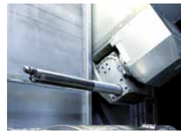
Drilling + ID boring
