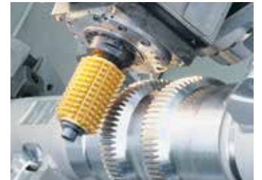
Hobbing of gear teeth (Flanx-Hob)
