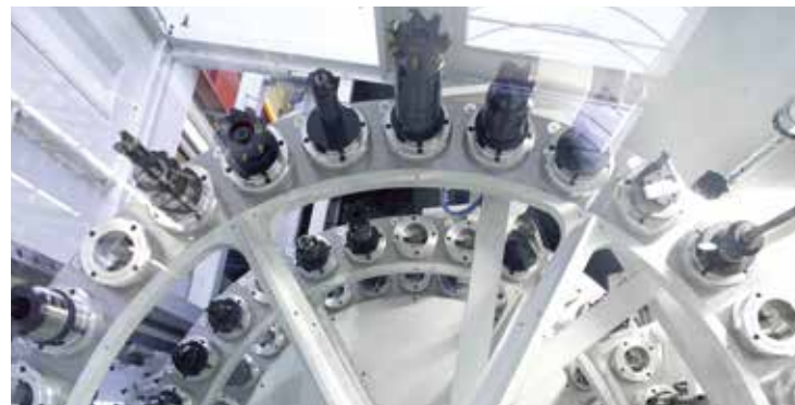
Maintenance-free disc magazine
