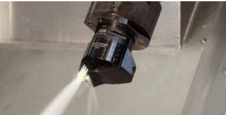
Ultra-High Pressure Coolant (UHPC)
