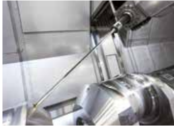
➤ Deep hole drilling
