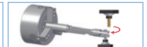
■ Increase work rigidity by PULL-Tension for Weak parts
