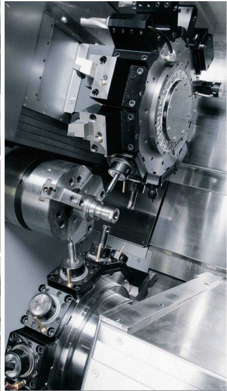
Simultaneous Milling with Upper and Lower Y-axes on Left spindle
