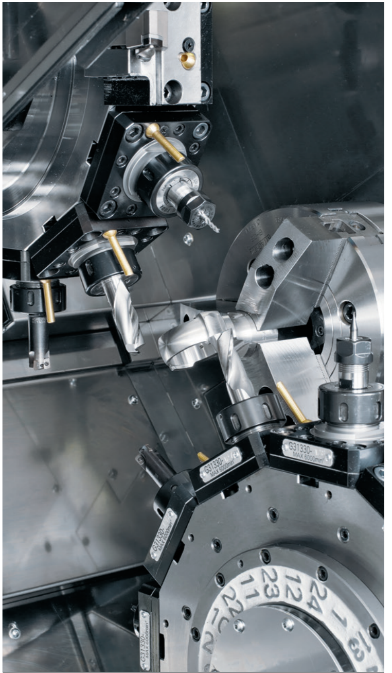
Simultaneous Milling with Upper and Lower Y-axes on Right spindle
