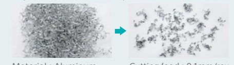
Material : Aluminum Cutting speed : 200mm/min
