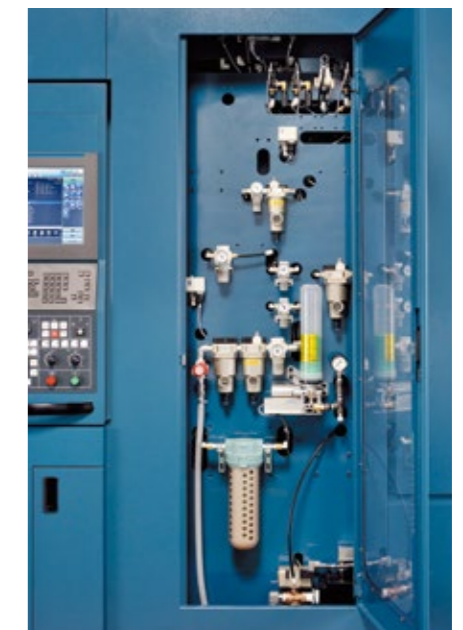
Centralized layout of maintenance devices
