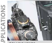
**ROLLING HEADS** It is possible to install them in a turret or as a unit dedicated and attached to the machine CIA bedframe. This application allows you to perform rolling operations directly on the Famar lathes, avoiding a secondary machining opũ eration. ۵.
