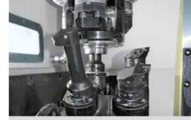
**MULTIPLE TOOLS** Specially designed, they eliminate turret rotation for passage from one tool to another, thus ensuring reduction in the cycle time.
