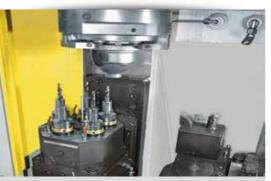
**MULTIPLE DEDICATED HEADS** Produced as a function of the workpiece, they are installed on the motor dedicated and fixed directly on the machine bedframe.
