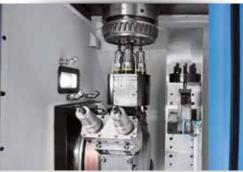
**MULTIPLE HEADS IN TURRET** Thanks to the torque performance and the power of Famar Turrets, it is possible to install multiple drilling and tapping heads directly on them, ensuring a significant reduction in cycle time.
