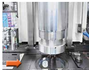
The spindle locks the piece
