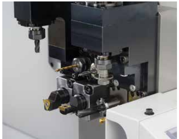
The back tool post on Type X and XII machines can accommodate a total of 8 tools: 4 rotary tools in the upper row and 4 fixed tools in the lower row.
