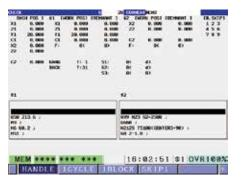
On-machine program check function Using manual hand feed, operations can be run in the forward or reverse directions, can be paused to edit the program, and restart.
