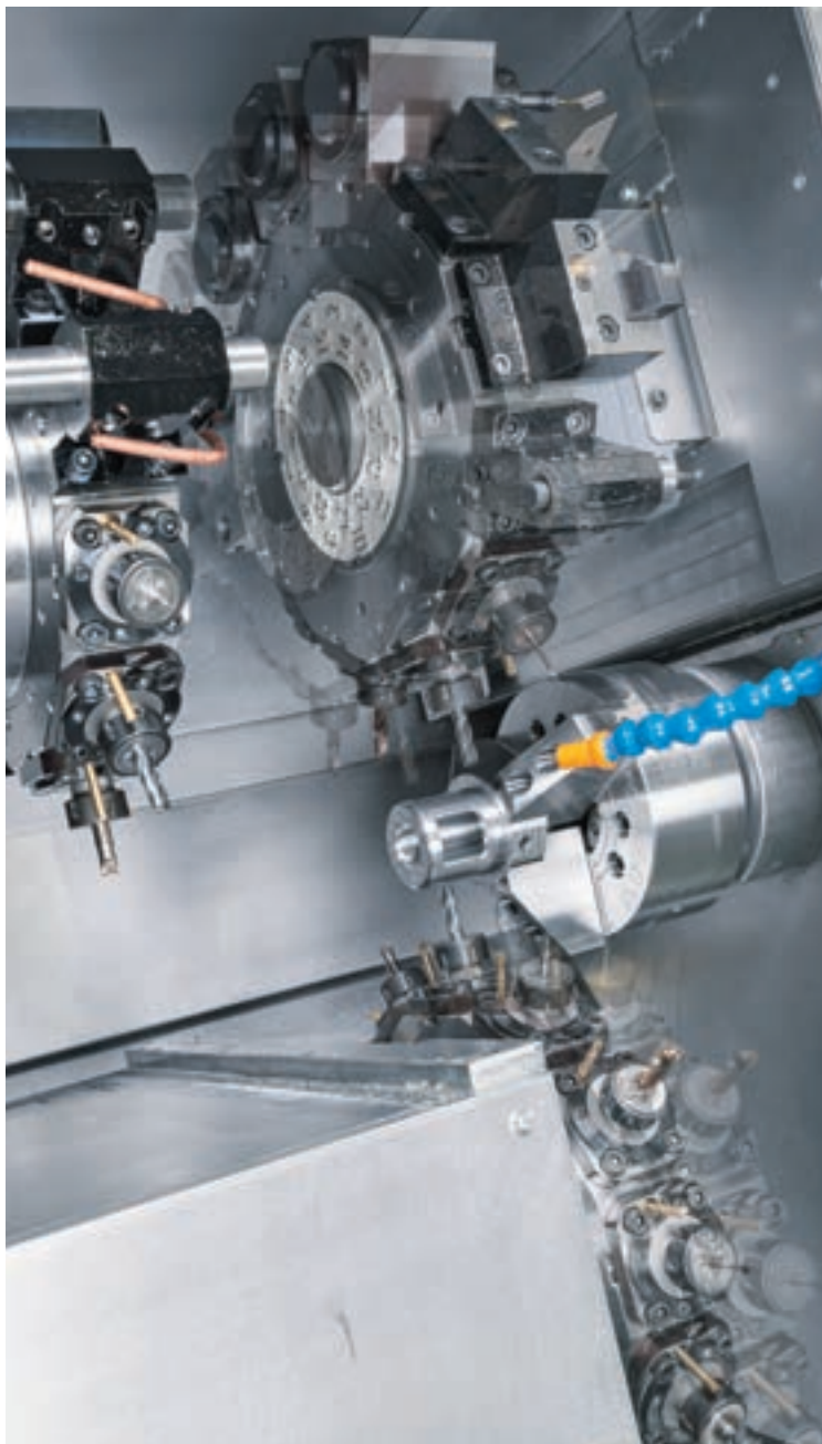
Simultaneous Milling with upper / lower tool on right spindle.
