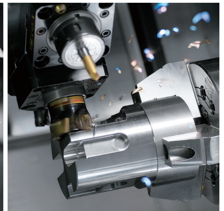
Dia. 50mm Face milling cutter Metal Removal Rate 148mL/min • Surface speed : 235m/min (1500min -1 ) • Depth : 4mm • Feed : 0.7mm/rev
