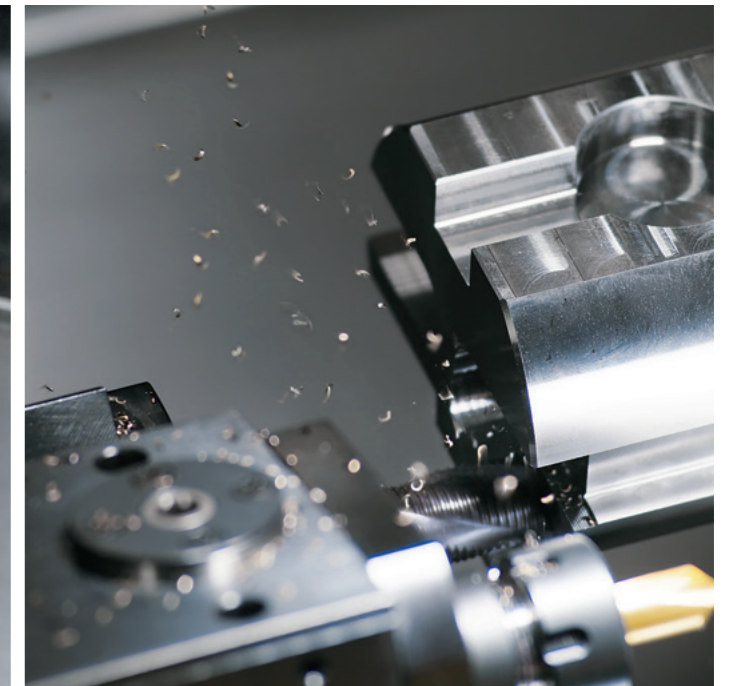
Dia. 20mm End mill Metal Removal Rate 34mL/min • Surface speed : 35m/min (557min -1 ) • Depth : 15mm • Feed : 0.2mm/rev
