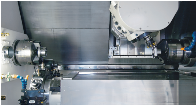
Milling with Tool Spindle on Right hand side Spindle, Machining with Lower Turret on Left hand side.
