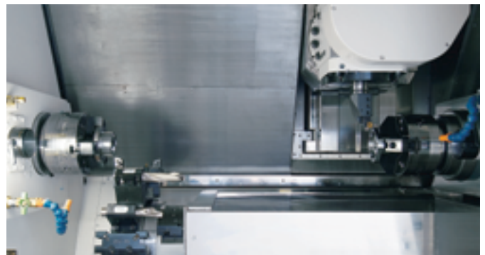
Turning with Tool Spindle on Right hand side, Lower Tool on Left hand side Spindle.
