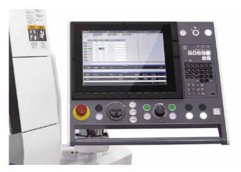
A 15-inch touch panel is adopted, and the new HMI (Human Machine Interface) enables intuitive operation.
