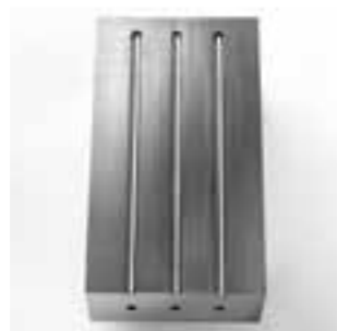
ø6 × 170mm (L/D=28) Workpiece: Carbon steel
