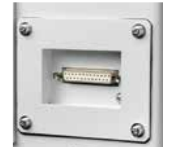
RS232C 25pin connector RS232C 25pin connector can be attached to the side of the control box.
