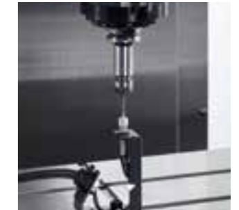
Tool breakage detector, touch type A touch switch type tool breakage detector is available.
