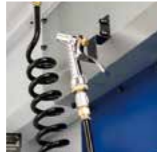
Cleaning gun Helps clean the workpiece or chips inside the machine after machining.
