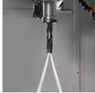
Coolant Through Spindle (CTS) Can be selected from 1.5 MPa or 7 MPa. Particularly effective in non-step peck drilling.
